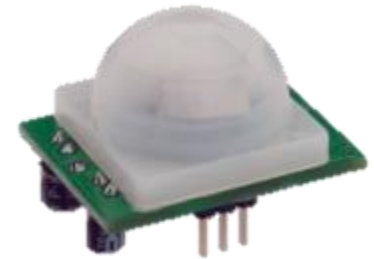
PIR* sensor *Passive infrared
