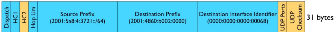
Compressed UDP/IPv6 Header (2001:5a8:4:3721:0217:3b00:1111:2222 → 2001:4860:b002::68)
