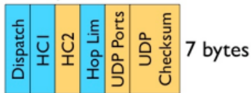
Compressed UDP/IPv6 Header (fe80::0217:3b00:1111:2222 → fe80::0217:3b00:3333:4444)
