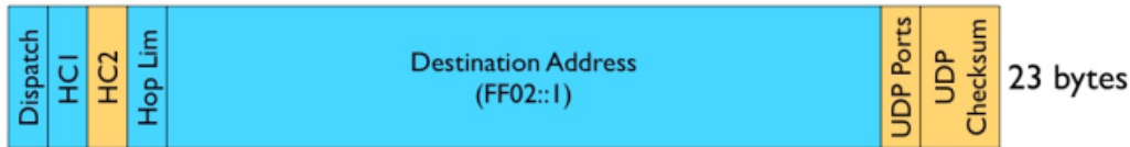
Compressed UDP/IPv6 Header (fe80::0217:3b00:1111:2222 → ff02::1)
