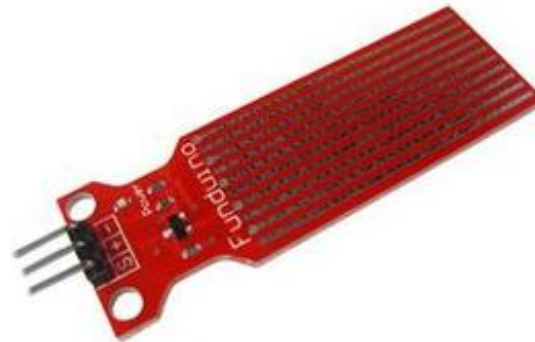
Water level sensor
